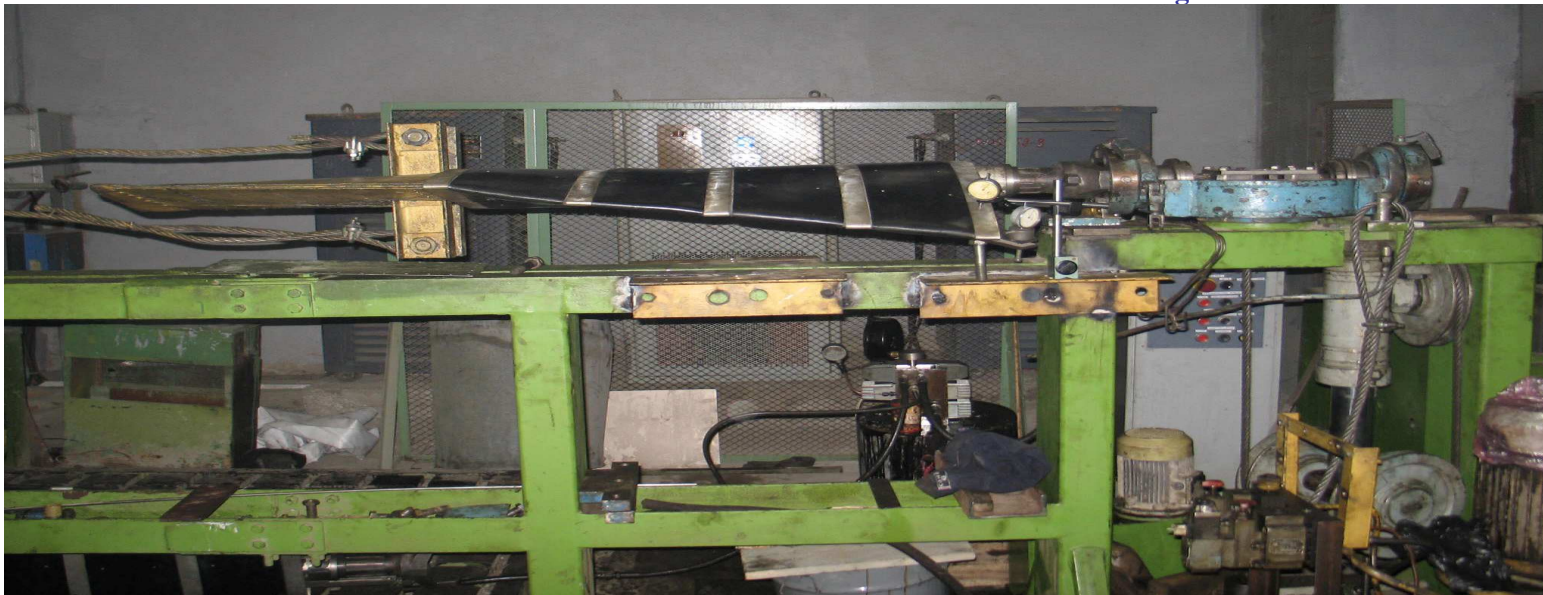
Blade with ribs without flexible elements on the stand for static investigations
