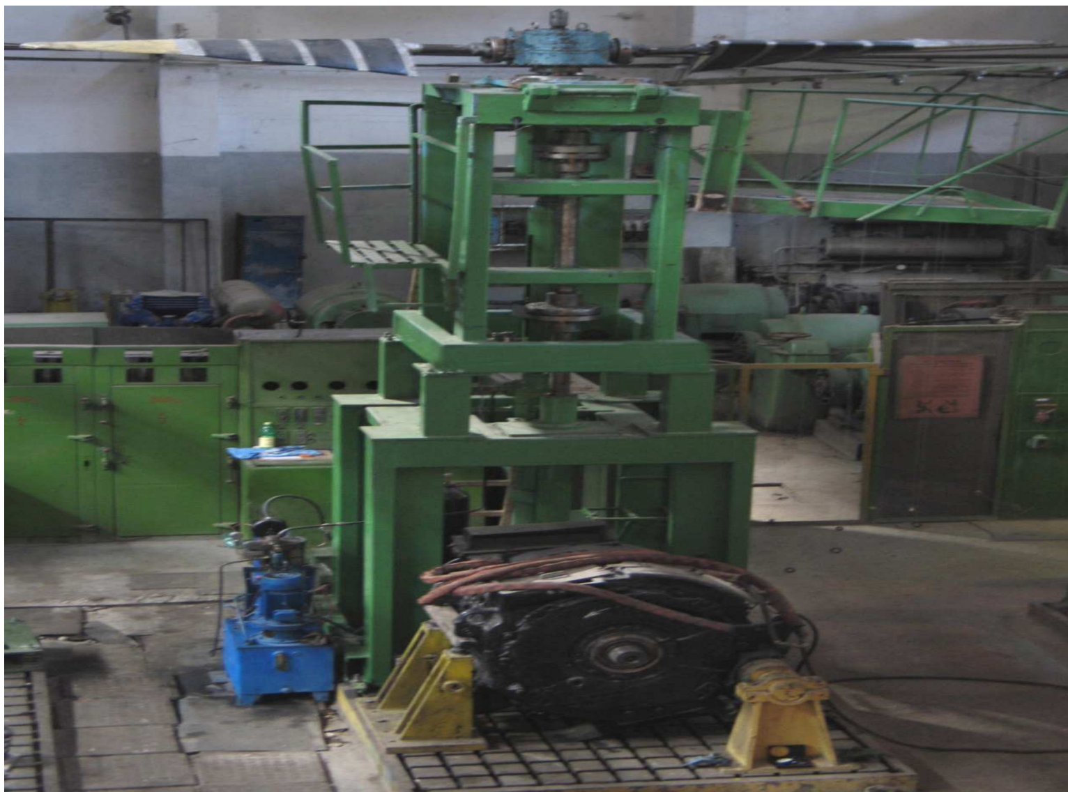
Project G-1600. Stand for dynamic tests of the VGR. Blades in retracted position.
