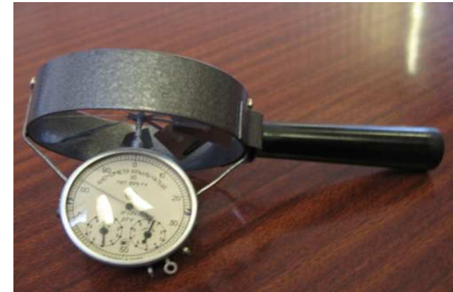
Revolving-vane analyzer ACO-3
