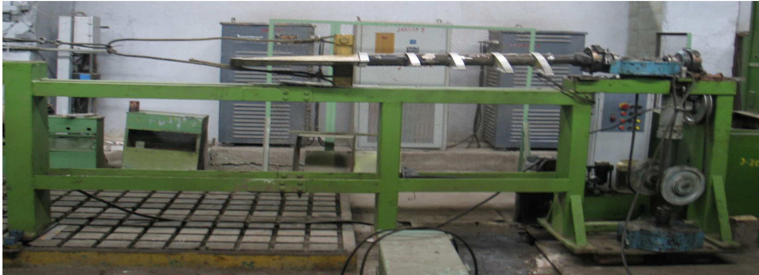
Blade with ribs without flexible elements on the stand for static investigations
